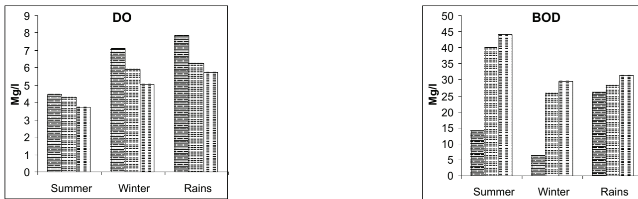
Figure - Seasonal variations of parameters in Wainganga river at water pumping station
