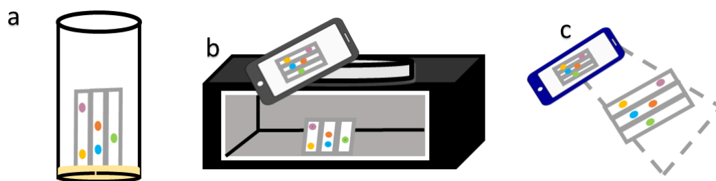
Figure 1 – a) Development of the TLC plates in the chromatographic chamber with a mobile phase system. b) Imaging through the eyepiece of a black box, c) direct imaging of the chromatographic plates.
